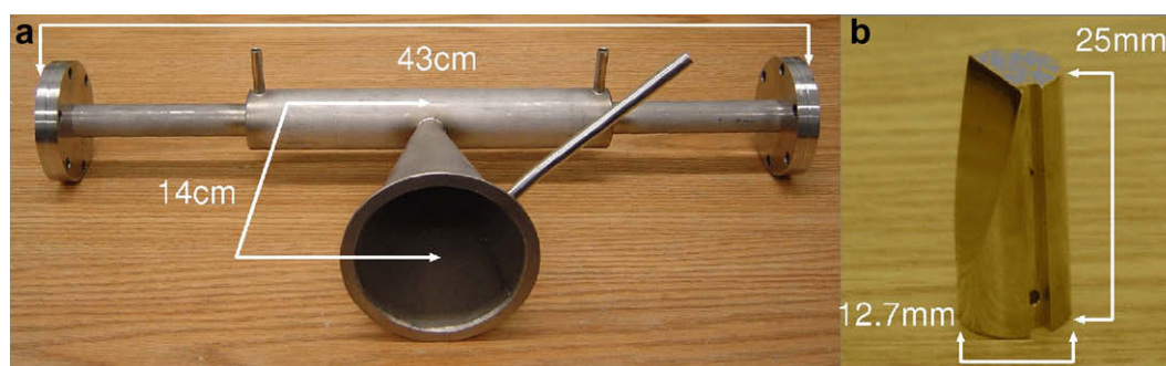
Fig. 1. High temperature furnace insert (a) and molybdenum rod sample with 15° angled side surface (b).
